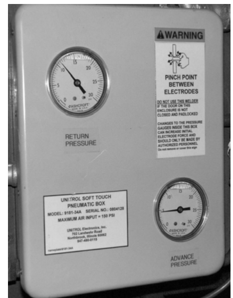
padlockable NEMA-12 regulator box
